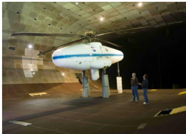
Figure 1.3: 4 bladed rotor in the NASA 40 by 80 Wind Tunnel
